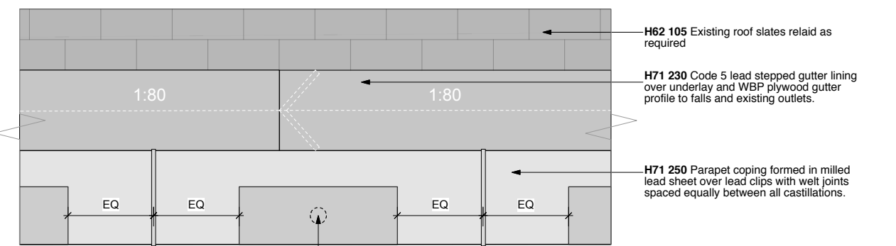
TROWTES HOUSE Typical Parapet plan 1:10 @ A1
